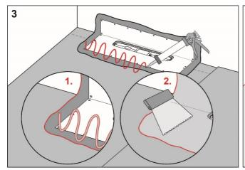
Apply PCI Pecitape Bond on the drain collar and PCI Lastogum to the rest of the floor and wall area.
