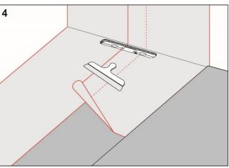
Install PCI Folie and overlap the drain collar by a minimum of 50 mm. Seal all seams with PCI Lastogum.
