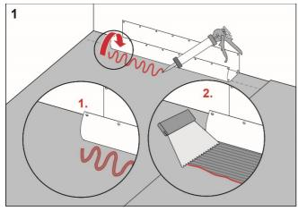
Apply PCI Pecitape Bond to the floor and wall areas which the drain collar will cover. Spread the adhesive with a fine-toothed adhesive spreader.
